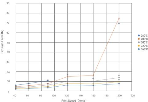
Test parameters: 12mm length brass heat block, BMG extruder, Hardened Steel Nozzle, Nozzle size 0.4mm, Layer Height 0.2mm
